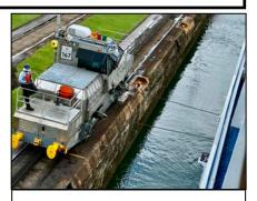
One of the four engines that pulled the ship through the Panama Canal
